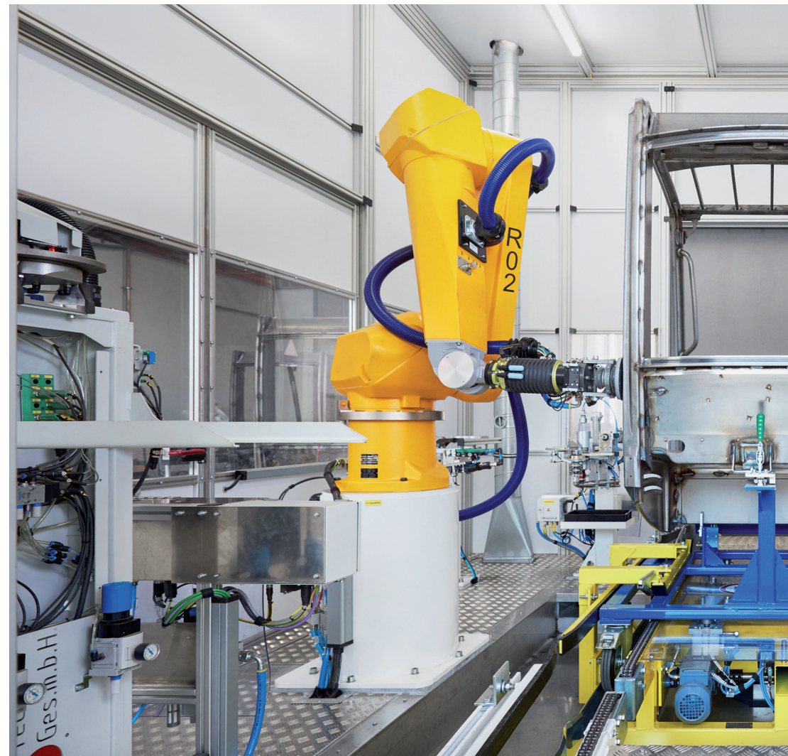
Full-automated grinding robot for cabin structures
