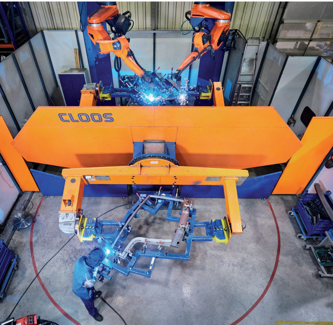
Welding robot for welding sub-groups e.g. side frames
