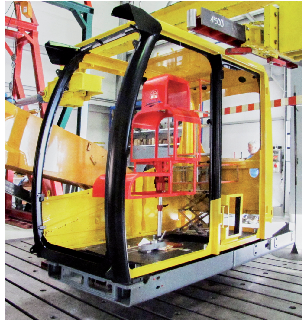
ISO tests for ROPS/FOPS safety structures
