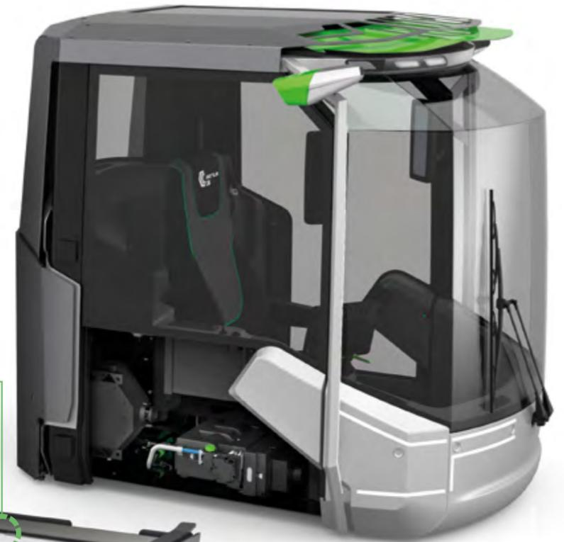
Modularer HYDAC CabinAirCare Filter
